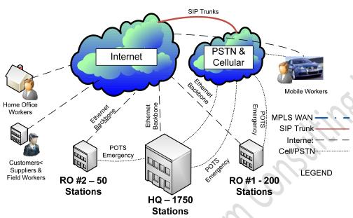
SIP trunks are terminated into the PSTN by the Ethernet IP Backbone provider at a discount to premise terminations (based on capacities, bulk rates and lower service costs). No PSTN access (except emergency access lines) terminated directly at each location.
