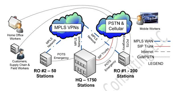
SIP Trunks between sites are converted to MPLS bandwidth. PSTN access over SIP trunks is centralized at HQ.
