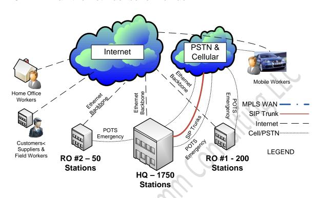
All communication, except for SIP trunks, is IP on Ethernet Backbone provider. PSTN access over SIP trunks is centralized at HQ.
