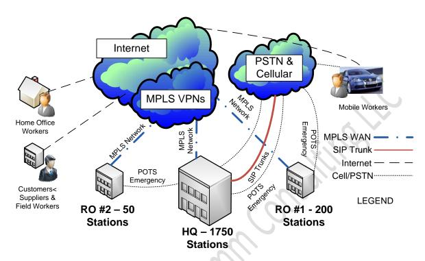
Remote users move to VoIP and Internet Protocol (for Unified Communications) reducing voice trunk usage (based on IM, presence and IP to remote workers, customers, & suppliers). Inter-site communications is still provided over MPLS with PSTN access over SIP trunks centralized at HQ.
